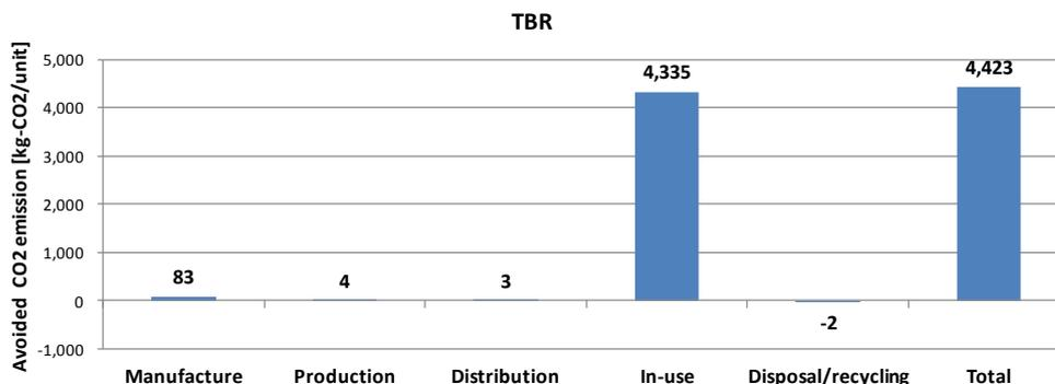
Fig.3 Avoided CO<sub>2e</sub> emissions per the automobile with PCR and TBR
