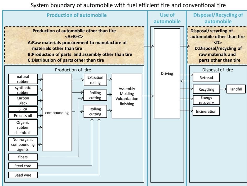
Fig.1. System boundary of automobile with fuel efficient tires and conventional tires
