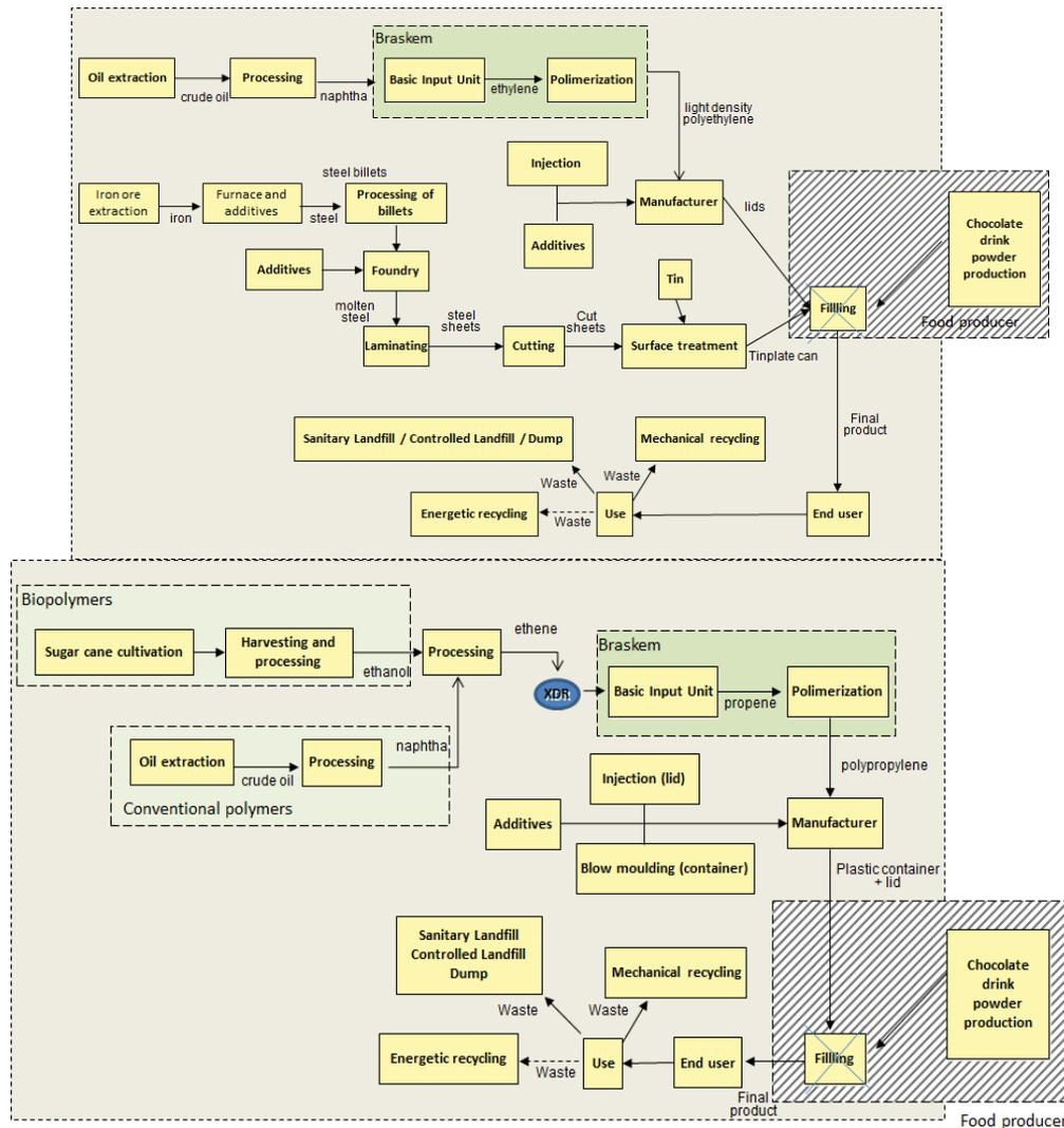
**Figure 2 - Flow-diagrams of the Polypropylene-based container system**
